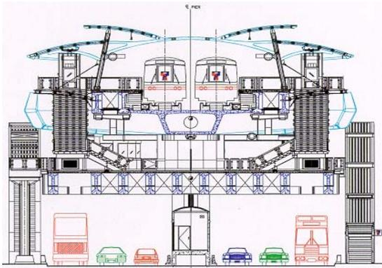
**Figure 7.** Cross section of a BTS station.
